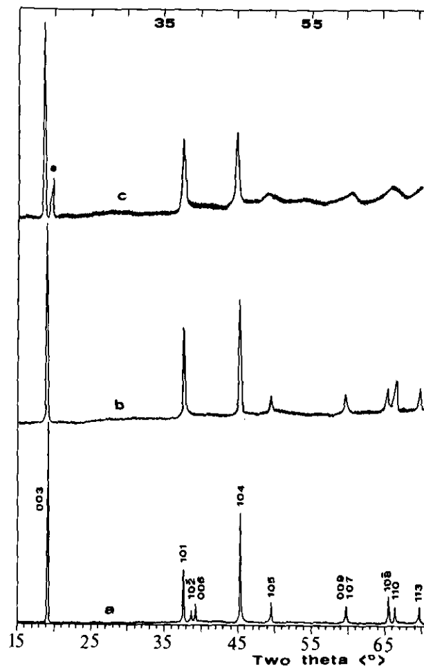
FIG. 1. X-ray patterns of LiCoO 2 (a), LiCoO 2 treated with 0.1 N H 2 SO 4 (b) and LiCoO 2 treated with 1 N H 2 SO 4 to a dissolution degree of 70% (c). The Miller indices of the Bragg peaks are indicated near each line. The circles denote the line with d = 4.50 Å not belonging to the initial XRD patterns.
